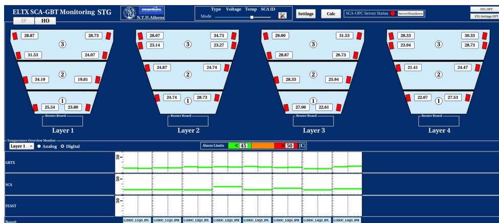
Figure 7.10: The SCA DCS panel for sTGC electronics monitoring.
