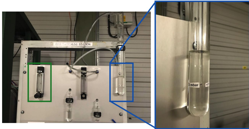
Figure 2.7: User turns left the gas INPUT flow-meter (green rectangle) until the gas bubble inside the pressure gas cylinder reach the black line of 3 mbar (blue rectangle).
