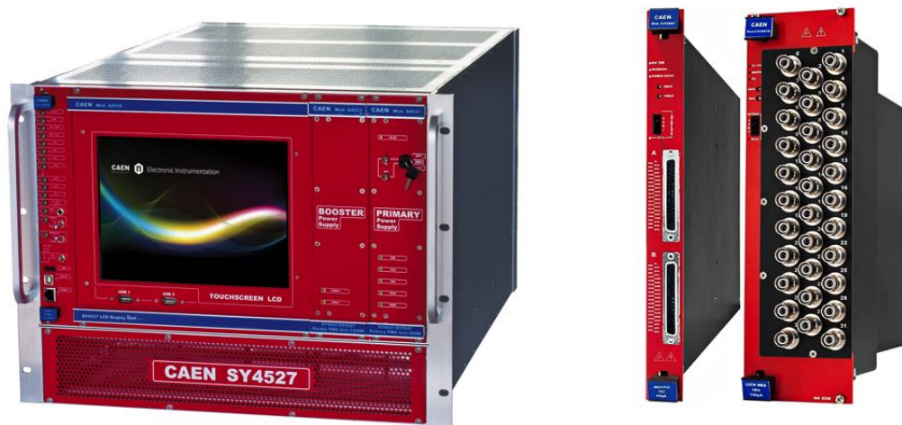
Figure 5.1: The CAEN mainframe SY4527 and CAEN HV boards A7038 with 32 channels which are commonly used for the Micromegas HV validation.
