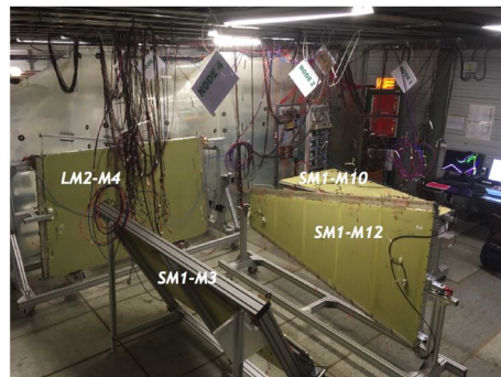
Figure 5.3: The Micromegas high voltage validation experimental setup at BB5.
